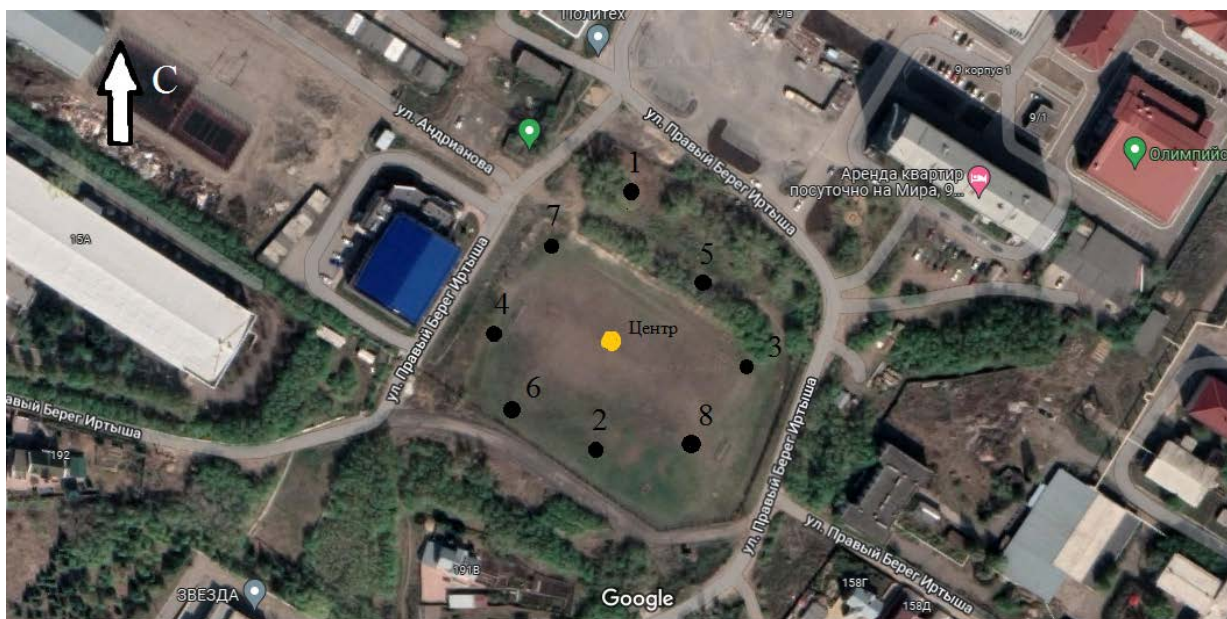
Figure 7 – Places for installing electrodes in open areas
